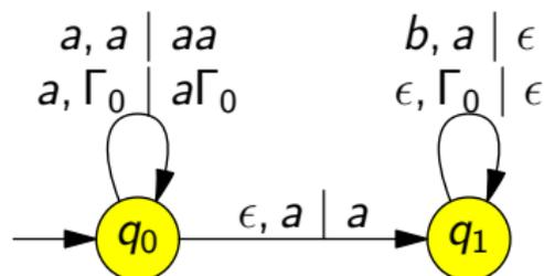
$$[q_0, \Gamma_0, q_1] \rightarrow a[q_0, a, q_1][q_1, \Gamma_0, q_1]$$
